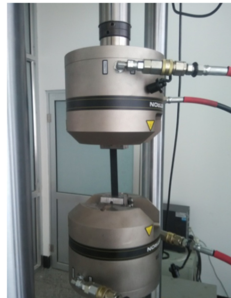
Fig. 3. Diagram of the servo-hydraulic testing system.
