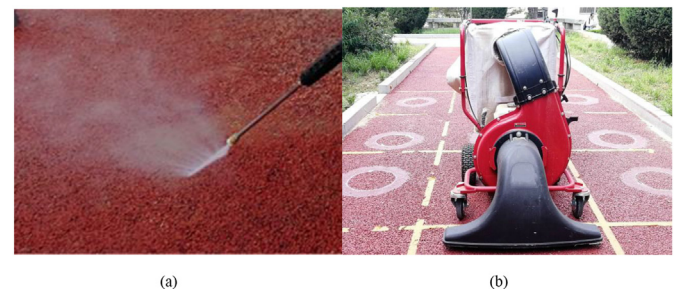
Fig. 5. Cleaning vehicle apparatus (a) Pressure washer, (b) Vacuum equipment.
