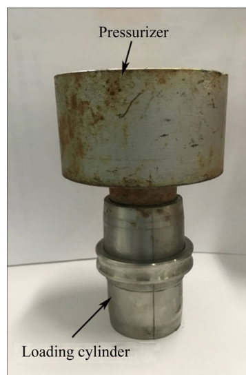
Figure 3 Photo of compacting apparatus
