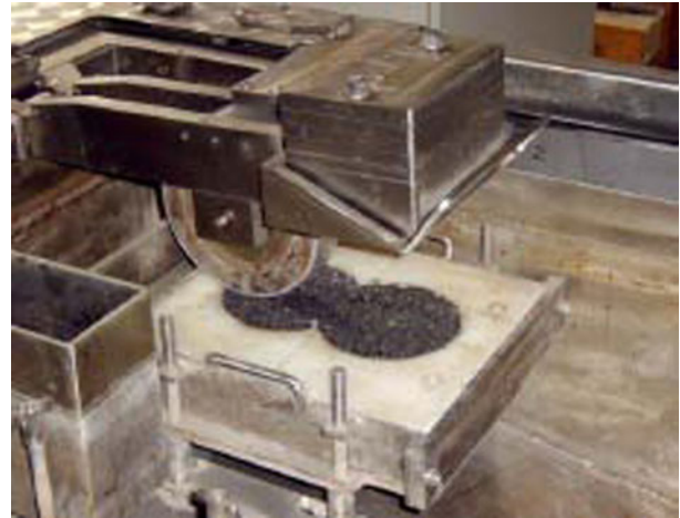
Figure 9. Assembly of specimen in HWTd test.
